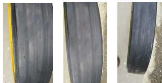
Figure 10: Photographs of developmental road wheel with NO FAILURES after 200 miles (80°F ambient track temperature at 40mph on YPG paved track)
