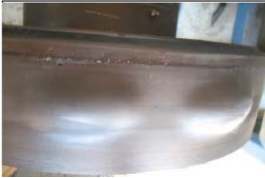
(a) Production RW – 48 min at 35 mph; 5500 lbf
