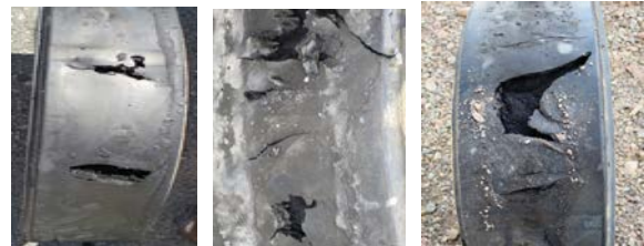
Figure 9: Photographs of production road wheel failure: hysteresis blow-out followed by chunking after only 20 miles (80°F ambient track temperature at 40mph on YPG paved track)
