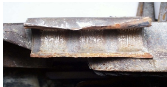
b) Track Block Rupture
