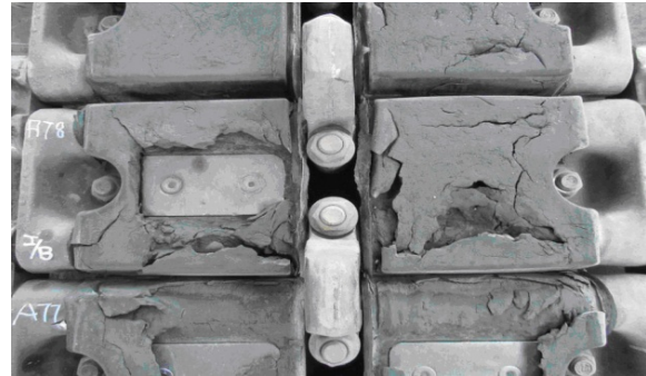
(b) Road Wheel Backer Pad (RWBP) Fatigue
