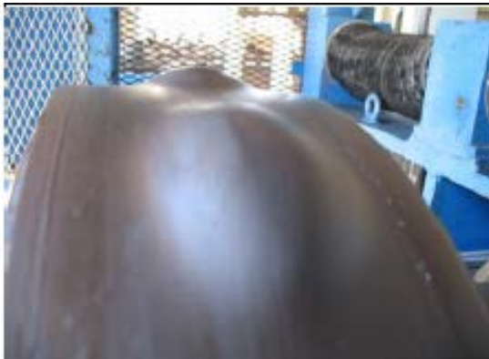
(b) Production RW – 46 min at 35 mph; 5500 lbf
