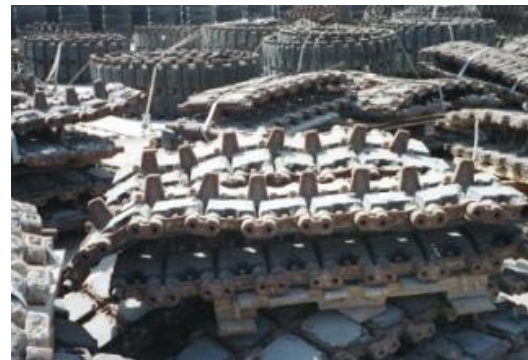
(a) Discarded track at ~ 740 miles
