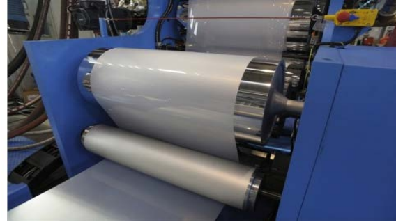
(c) Calendaring uncured rubber stock for tire building and curing
